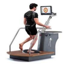
Postural stability is evaluated using a stabilometric platform known as the TecnoBody ProKin (Figure 1), a force platform designed to measure postural sway by analyzing the center of pressure (Toprak et al., 2019).
